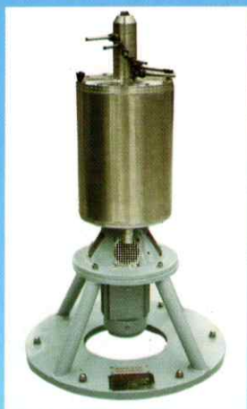
PILOT PLANT EXTRACTOR 6-stages Bowl Ø 120 mm flowrate 10 to 30 l/hr
