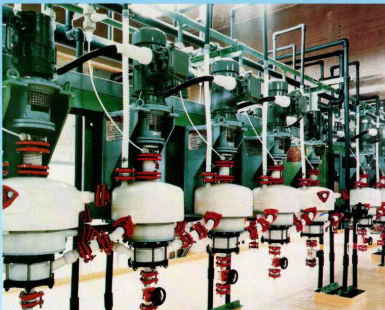
SERIES OF MONOSTAGE EXTRACTORS - Solid PVDF construction Bowl : Ø 360 mm - Flowrate : 12 m 3 /hr
